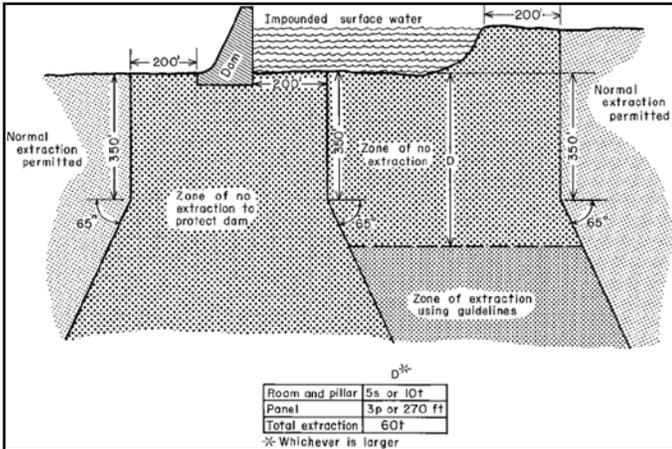
Figure 4. Embankment and basin safety zones of an impoundment (Babcock et al., 1977).
