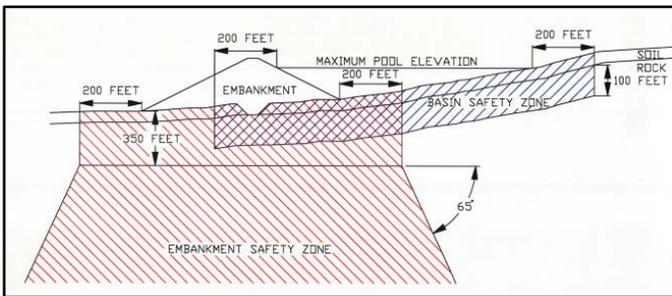
Figure 5. Schematic of impoundment embankment and basin safety zones delineated in the West Virginia dam safety regulations.
