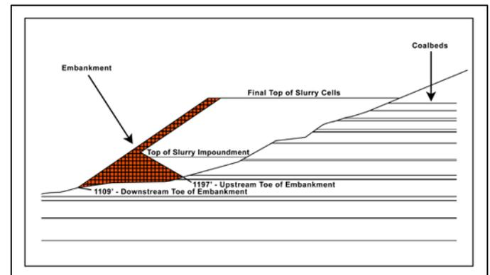
Figure 6. Schematic longitudinal profile of an impoundment in West Virginia showing multiple coal seams adjacent as well as subjacent to the facility.
