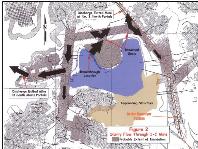
**Figure 3.** Illustration of the October 11, 200 breakthrough at the Big Branch coal waste slurry impoundment in Martin County, KY (modified from MSHA, 2001).
