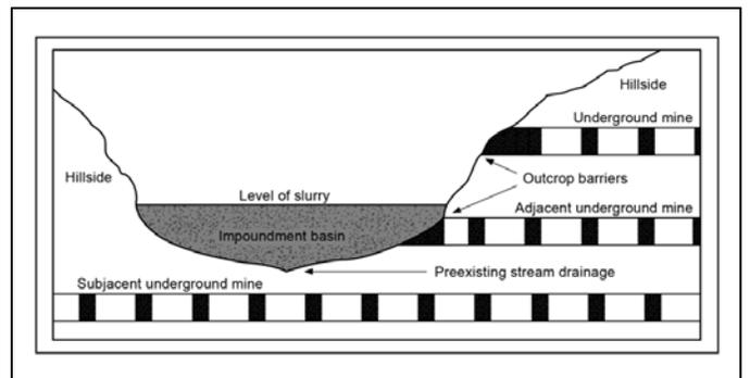
**Figure 2.** Schematic cross section of an impoundment basin and adjacent and subjacent underground mines in the bituminous Appalachian coal fields (modified from the NRC, 2002).
