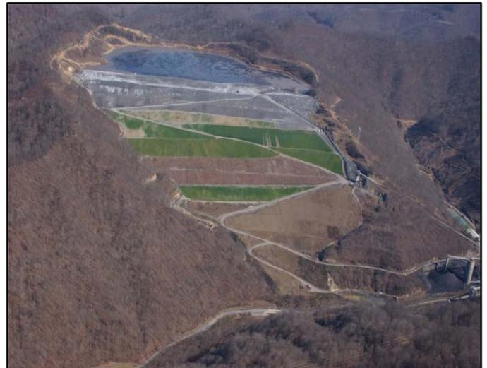
**Figure 1.** Example of a coal waste slurry impoundment in steep-slope topography in West Virginia.
