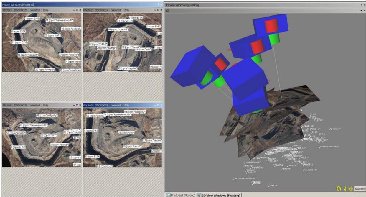
**Figure 6** March amateur photos oriented with survey points.
