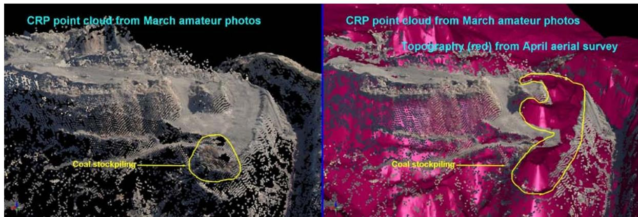
**Figure 9** March and April coal stockpiling compared.
