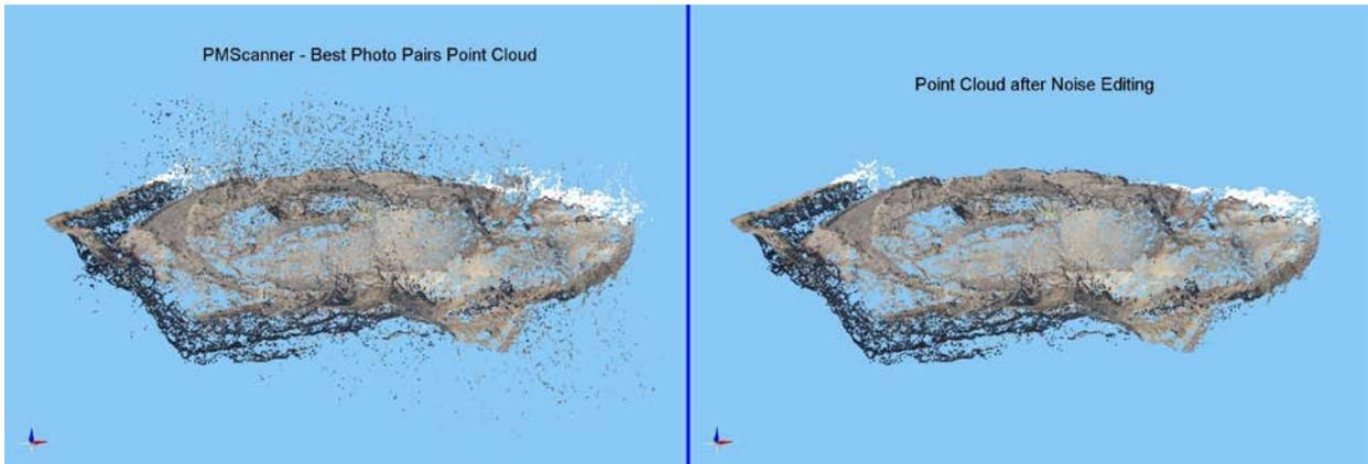
**Figure 7** CRP Point cloud from amateur photos.
