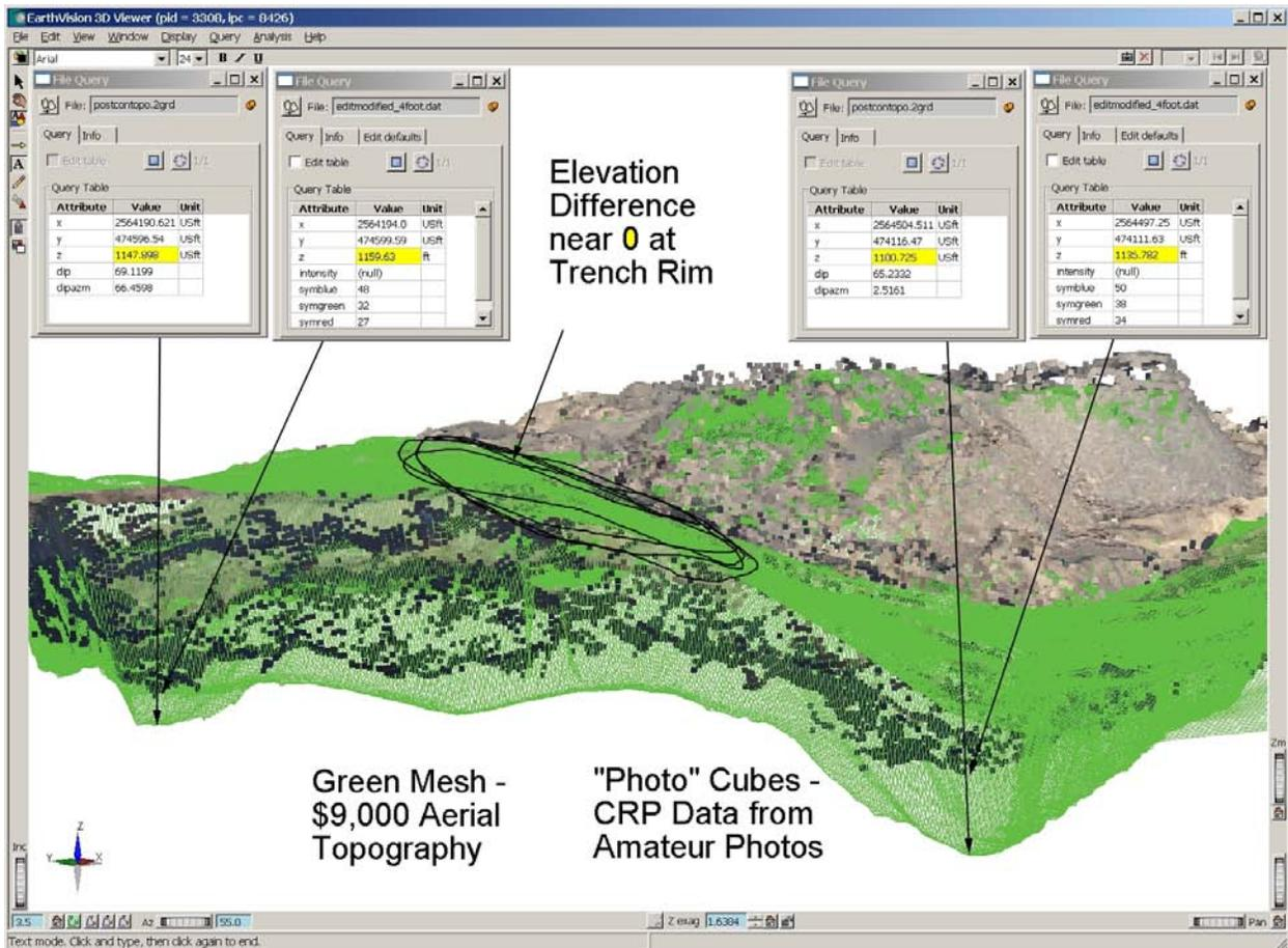
Figure 8 CRP point cloud compared with Aerial Survey.
