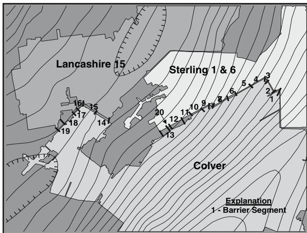
**Fig. 3** Saturated coal barrier between the Colver, Lancashire 15, and Sterling 1 and Sterling 6 mines
